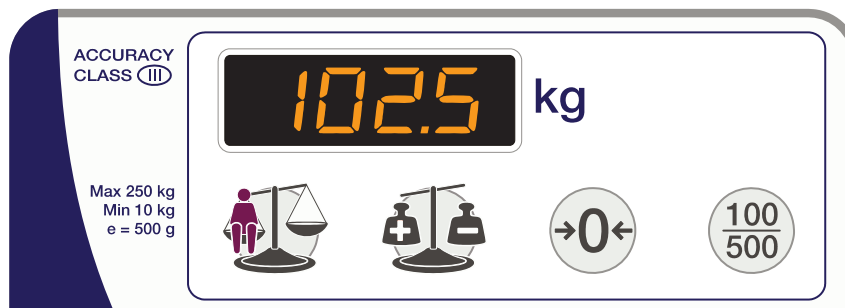
Fig. 21 - Patient weighing system controls
